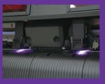
Applies UV-curable ink that hardens immediately through irradiation of ultraviolet (UV) light
